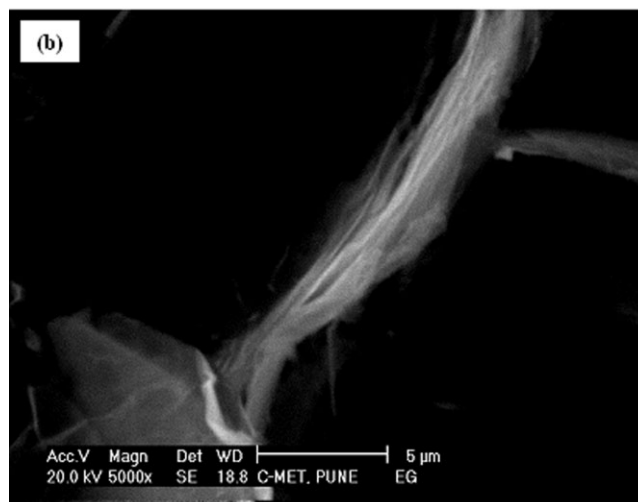
Figure 4 SEM of EG powder at scale bar (a) 20\text{ }\mu\text{m} and (b) 5\text{ }\mu\text{m} .
